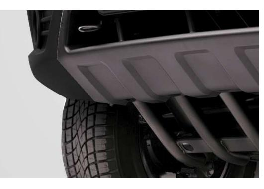
The steering rod protection will keep units placed low to the ground intact when hitting an obstacle. The protection is made of 42-mm steel tubes. Its design is stiff enough to protect the steering rods.
