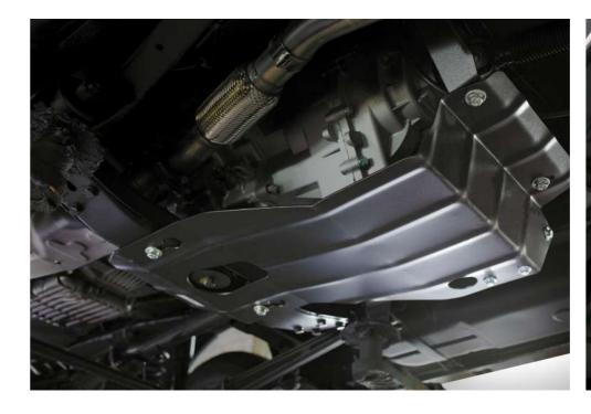
The steel sheet metal protects the most important vehicle units: the gearbox and and the transfer. The protection is set apart by its strength, corrosion resistance and reliable attachments.
