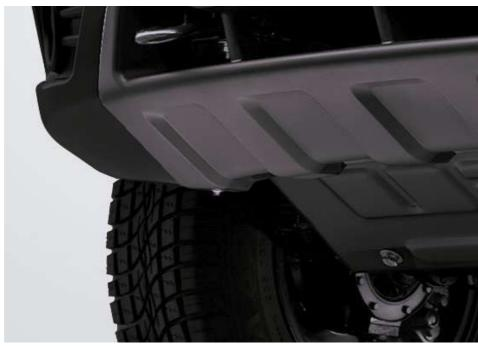
The steering rods will stay safe when hitting an obstacle. The protection is made of 3-mm steel sheet metal. Its design features high impact resistance.
