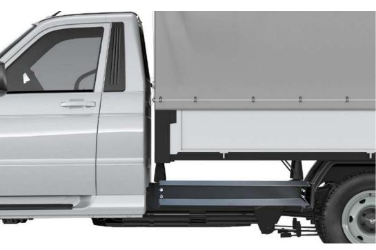
The underrun bar reduces the risk of serious injury to the drivers and passengers in the event of a road accident. The bar is made of two halves. Each half includes a beam attached to the vehicle frame with two energy absorbing brackets.
