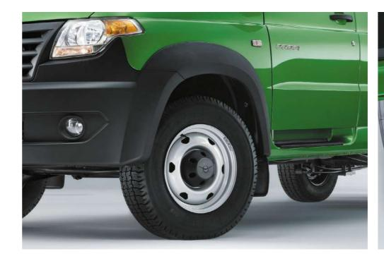
These plastic fender liners protect the wheel wells from corrosion. Your wheel wells will be able to weather even the most severe of vehicle operation conditions.
