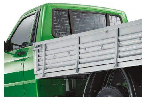
The grid provides glass protection when transporting cargo and gives extra protection when transporting long objects. And it does not affect visibility from the driver seat.
