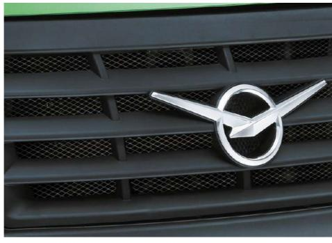
The grid protects the radiator from damage and clogging with foreign particles, thus preventing the engine from overheating. The grid cells size both ensures reliable protection and does not interfere with air flows.
