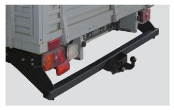
The tow hitch is designed to provide articulated coupling between the vehicle and the trailer. It is developed in accordance with the vehicle design features.
