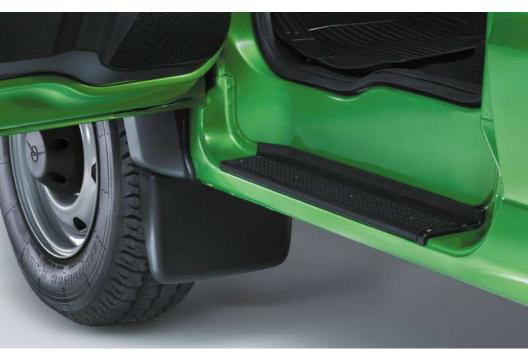
The mudguards are perfectly matched to your vehicle size, easy to install and very practical. They protect the body from chips and mud both in urban environment and off-road conditions.
