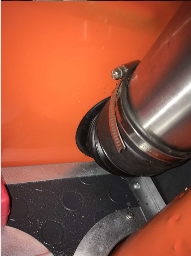
The pipe is entering the separation wall behind passengers seat and than entering the engine compartment.
