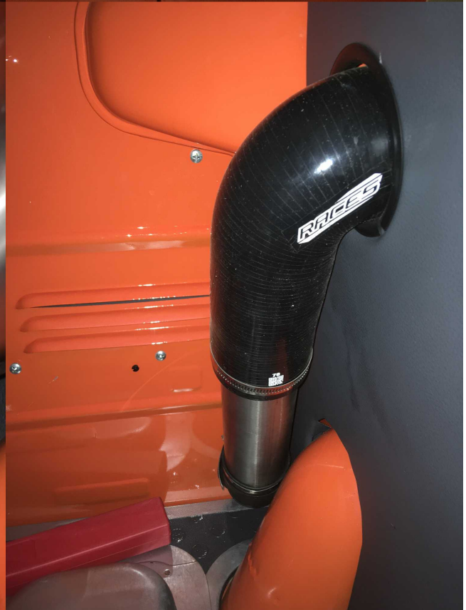
The pipe is entering the separation wall behind passengers seat and than entering the engine compartment.
